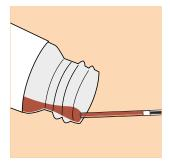
Tilt the control vial slightly. Place the capillary just below the control surface. Fill the blue striped capillary with the sample up to the white stopper. The control is stable for 5 minutes in the capillary.
