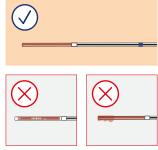
Note! Do not place the capillary to the bottom of the vial. If there are air bubbles on the capillary, discard it and collect a new sample. Wipe away any residual sample from the outside of the capillary.
