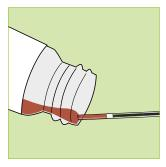
Tilt the control vial slightly. Place the capillary just below the control surface. Fill the orange striped capillary with the sample up to the white stopper. The control is stable for 5 minutes in the capillary.
