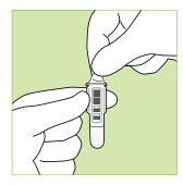
Remove the foil cover from the cuvette.
