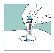
Choose Quality Control on the screen of the QuikRead go instrument. Insert the cuvette into the measurement well of the instrument. The barcode should be facing you.
