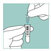
4 Insert the sample collector into the cuvette within 2 minutes.
