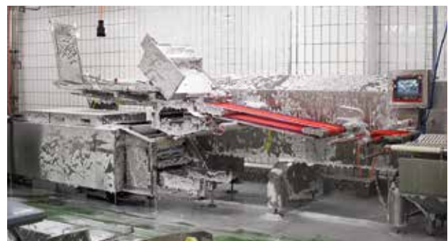
Equipment is washed carefully, and the result is checked with Hygicult TPC.
