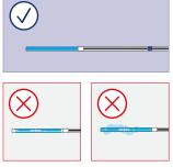
Note! Do not place the capillary into the foam. If there are air bubbles on the capillary, discard it and collect a new sample. Wipe away any residual sample from the outside of the capillary.
