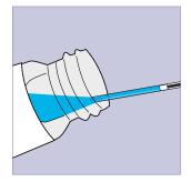
Tilt the control vial slightly. Place the capillary just below the control surface. Fill the blue striped capillary with the sample up to the white stopper.
