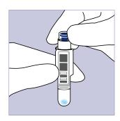
Close the cuvette tightly with the blue reagent cap. Do not press down the coloured inner part of the reagent cap. Perform the test within 15 minutes.
