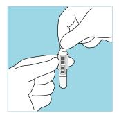
Remove the foil cover from the cuvette. Do not touch the clear flat surfaces in the lower part of the cuvette.
