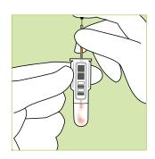
Place the sample (10 μl) into the buffer solution in the cuvette and dispense by pressing down the plunger. Make sure that the capillary is completely empty.
