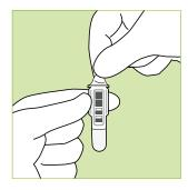
Remove the foil cover from the cuvette.
