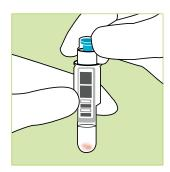
Close the cuvette tightly with the turquoise reagent cap. Do not press down the coloured inner part of the reagent cap. Perform the test within 2 hours.
