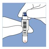
Close the cuvette tightly with the blue reagent cap. Do not press down the coloured inner part of the reagent cap. Perform the test within 2 hours.
