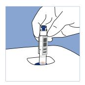
6 Insert the cuvette into the measurement well of the instrument. The barcode should be facing you.
