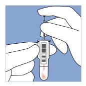
Place the sample (20 μl) into the buffer solution in the cuvette and dispense by pressing down the plunger. Make sure that the capillary is completely empty.
