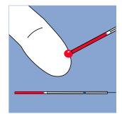
Pill the blue striped capillary with the sample (20 μl) up to the white stopper. Ensure that there are no air bubbles in the capillary. Wipe away any residual sample from the outside of the capillary.
