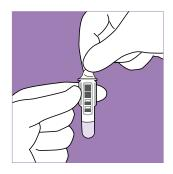
Remove the foil cover from the cuvette. Do not touch the clear flat surfaces in the lower part of the cuvette.
