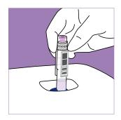
Choose Measure / Measure sample on the screen of the QuikRead go instrument. Insert the cuvette into the measurement well of the instrument. The barcode should be facing you.
