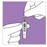
Insert the sample collector into the cuvette within 1 minute. The sample collector does not touch the solution in the cuvette.
