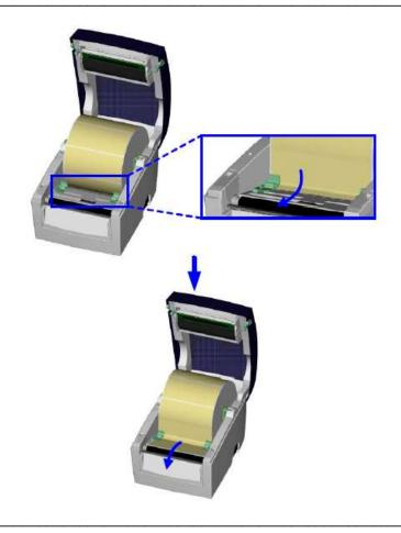
8. Adjust the paper guides to the width of label printer.
