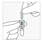
**4** Insert the sample collector into the cuvette within 2 minutes.
