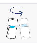
2 Mix the control vial gently by swirling. Do not shake to prevent foaming! In case a film appears on top of the vial, wait until it bursts or carefully remove it with a corner of lint-free paper. Keep the bottleneck clean.
