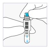
**5** Close the cuvette tightly with the easy CRP reagent cap. Do not press down the turquoise inner part of the reagent cap. Perform the test within 15 minutes.
