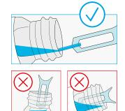
**3** Tilt the control vial until the control solution reaches the bottleneck. Place the sample collector almost horizontally just below the control surface at the mouth of the vial. Fill the capillary part of the sample collector completely.
