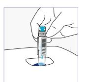
6 Choose Quality control on the display of the QuikRead go Instrument. Insert the cuvette into the measurement well of the instrument. The barcode should be facing you.
