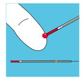
2 Fill the orange striped capillary with the sample (10 µl) up to the white stopper. Ensure that there are no air bubbles in the capillary. Wipe away any residual sample from the outside of the capillary.
