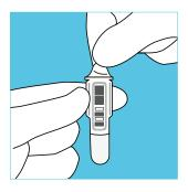
Remove the foil cover from the cuvette.
