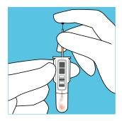
Place the sample  $(10 \ \mu l)$  into the buffer solution in the cuvette and dispense by pressing down the plunger. Make sure that the capillary is completely empty.
