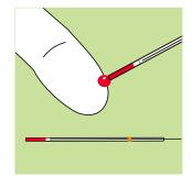
2 Fill the orange striped capillary with the sample (10 µl) up to the white stopper. Ensure that there are no air bubbles in the capillary. Wipe away any residual sample from the outside of the capillary.
